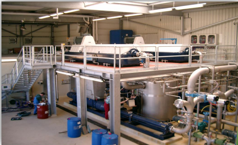
centrifuge with pipe system and thick material pump
